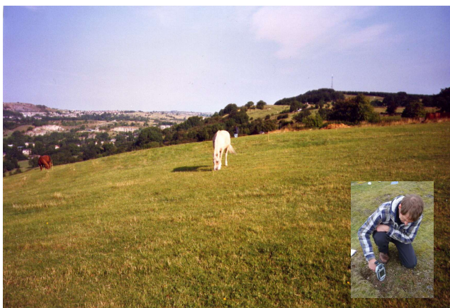
Site of a medieval Pb smelter at Wirksworth, Derbyshire, UK Hand-held portable x-ray fluorescence spectrometer (PXRF) used to measure Pb concentration [Pb] in topsoil in situ *
