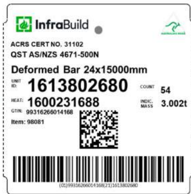
Figure 4. InfraBuild steel bundle data embedded barcodes example
